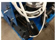
Whenever you disconnect the sprayer, be sure to put dielectric grease on all connections and make sure they are covered to avoid exposure to the elements.
