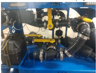
3. Self-Fill Mode - Your valves need to be in this configuration when you are using the pump on your sprayer to self fill from a holding tank.
