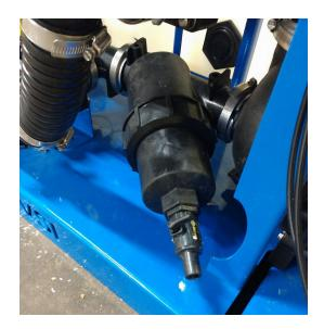
Each sprayer is equipped with a filter. Inside is a stainless steel 30 mesh filter that is reusable. Loosen collar around filter around housing and pull outer housing off and remove filter. Rinse clean and place back in the housing. The valve on the end of the filter housing is for a "quick clean" option when in the field. With the tank valve open and the pump running, open valve to blast debris out of the housing.
