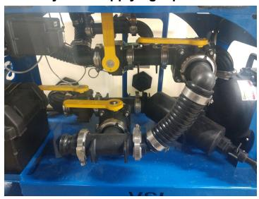
2. Pump-Out Mode - Your valves need to be in this configuration when you are using the pump to transfer liquid from the sprayer to another tank outside of the sprayer.
