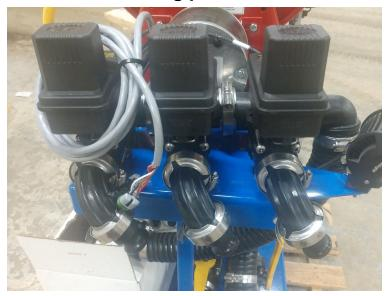
LEFT: Driver side 3 Lane, #1 on controller CENTER: Middle boom, #2 on controller RIGHT: Passenger side 3 Lane, #3 on controller
